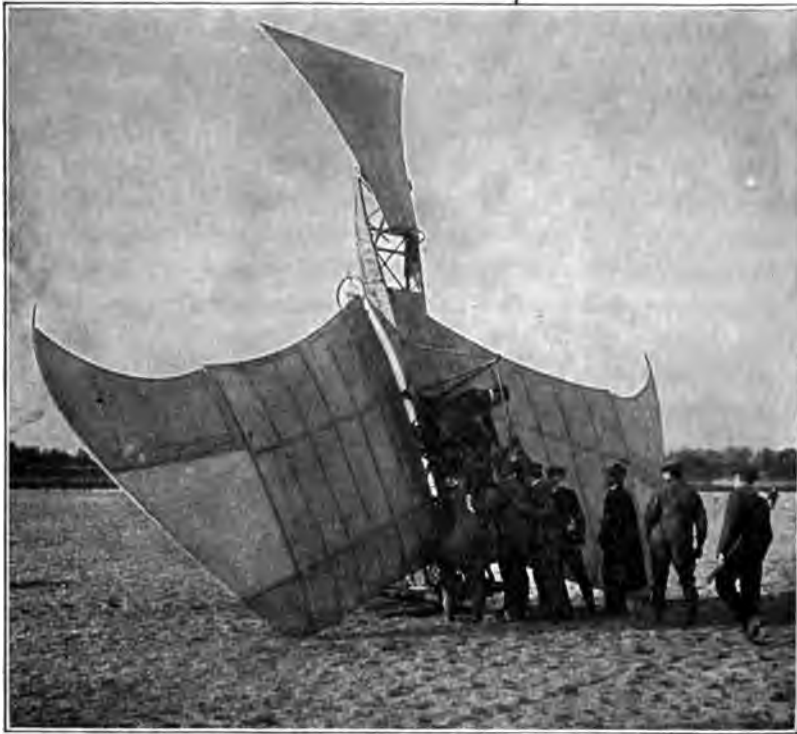
Fig. 49. Monoplane is Liable to Stand on its Head if Landing is Not Properly Made
